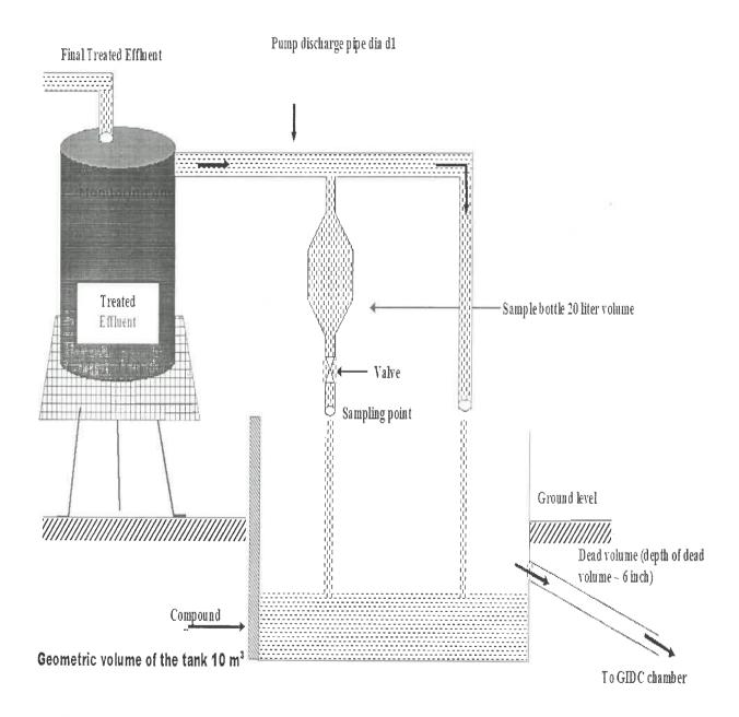
Note d1: Diameter of the discharge line should be such that it can not allow discharging the daily flow in a shorter duration say 2 – 3 hrs. Daily discharge strictly as per CCA, should take at least 18 – 22 hrs a day
